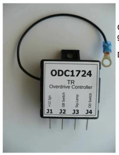
Connect the free wire (black) to the ground (chassis ground).
