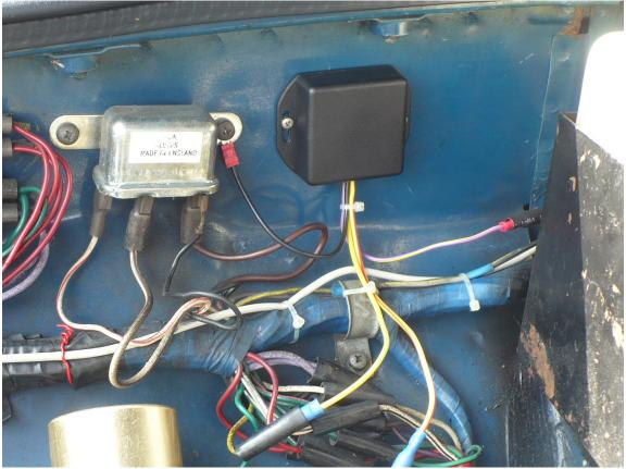
Connect the Black ground wire to chassis ground, existing mounting screw or extra drilled hole. Make sure it is not isolated by paint.
