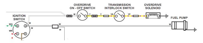
The ODC is connected between the OVERDRIVE ON-OFF SWITCH (Yellow wire) and the (Yellow-Red) wire connected to the TRANSMISSION INTERLOCK SWITCH. The 2 wires are connected by a bullet on the right side in the engine compartement. Look for this bullet. Disconnect the two wires and let the bullet connector left on the yellow wire.
